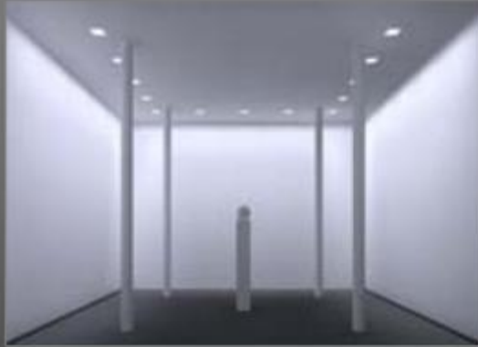
walls lit with grazing fixtures
